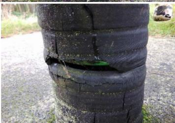
Finding: The spring cover is damaged, split or missing
